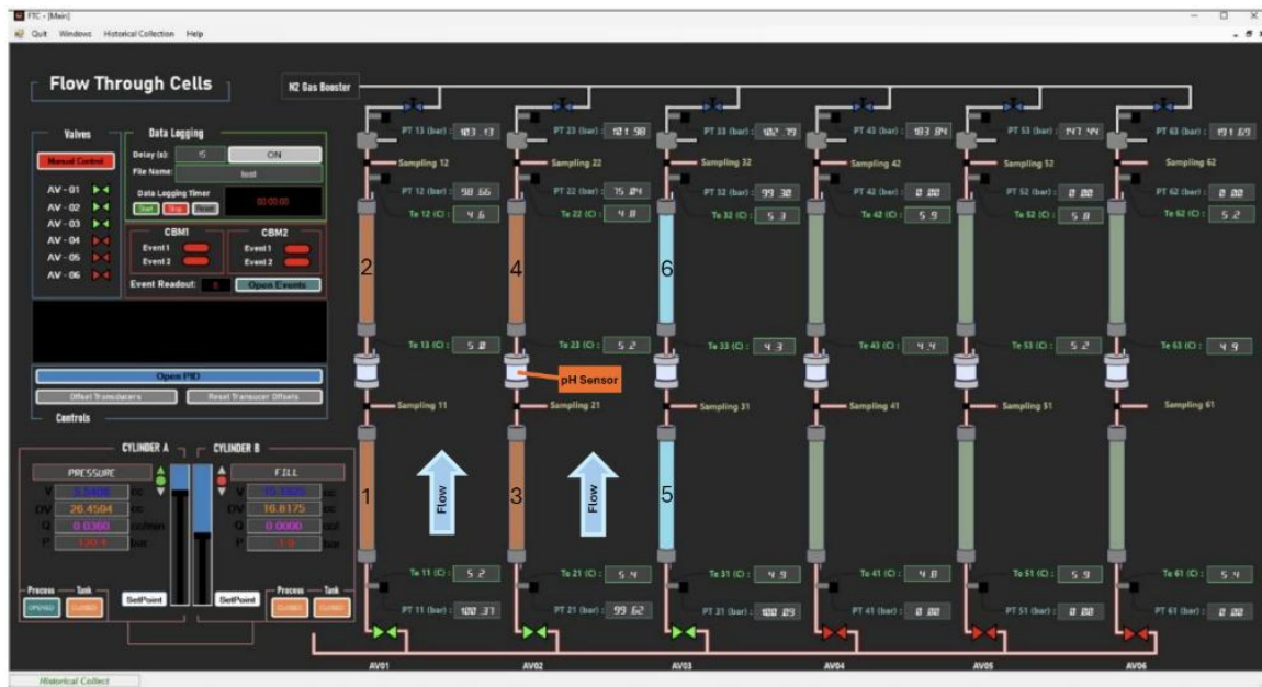
Figure 10. Configuration of sandpicks (brown for sediment-containing SP & blue for control SP), pH sensor (orange), and flow direction (blue arrows) in the Vinci software interface
