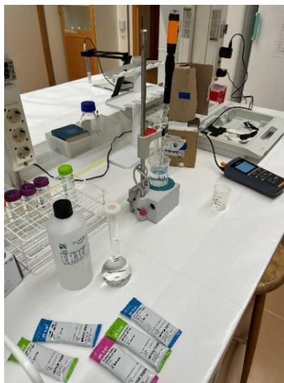
Figure 19. Calibration of the pH meter and measurement of prepared solution pH
