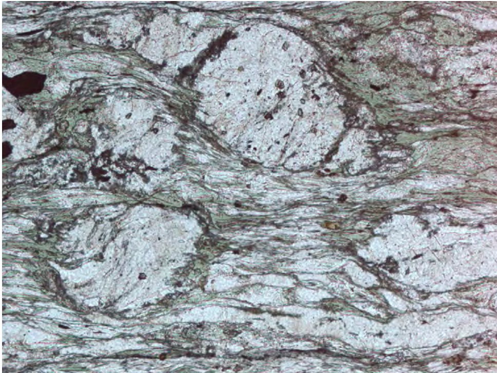
Figure 50: Thin section 5: Plane-polarized light (PPL), 5× objective, Albit (twin), white mica, chlorite.
