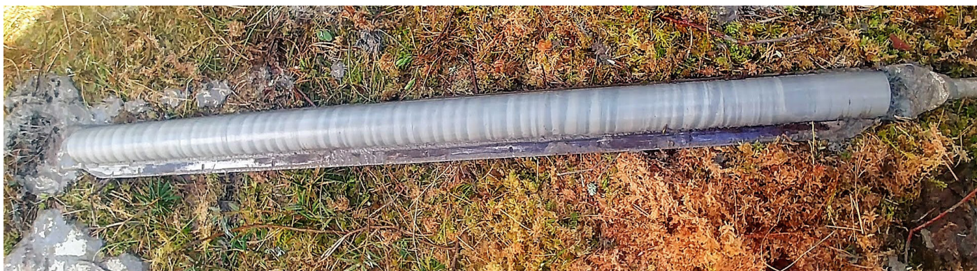
Core with glacial clay varves, from Lundinsmossen, Sörmland. This bog has been used for several courses on both Bachelor and Master's level. We analyse cores in the Sediment Laboratory. Photo: Stefan Wastegård.
