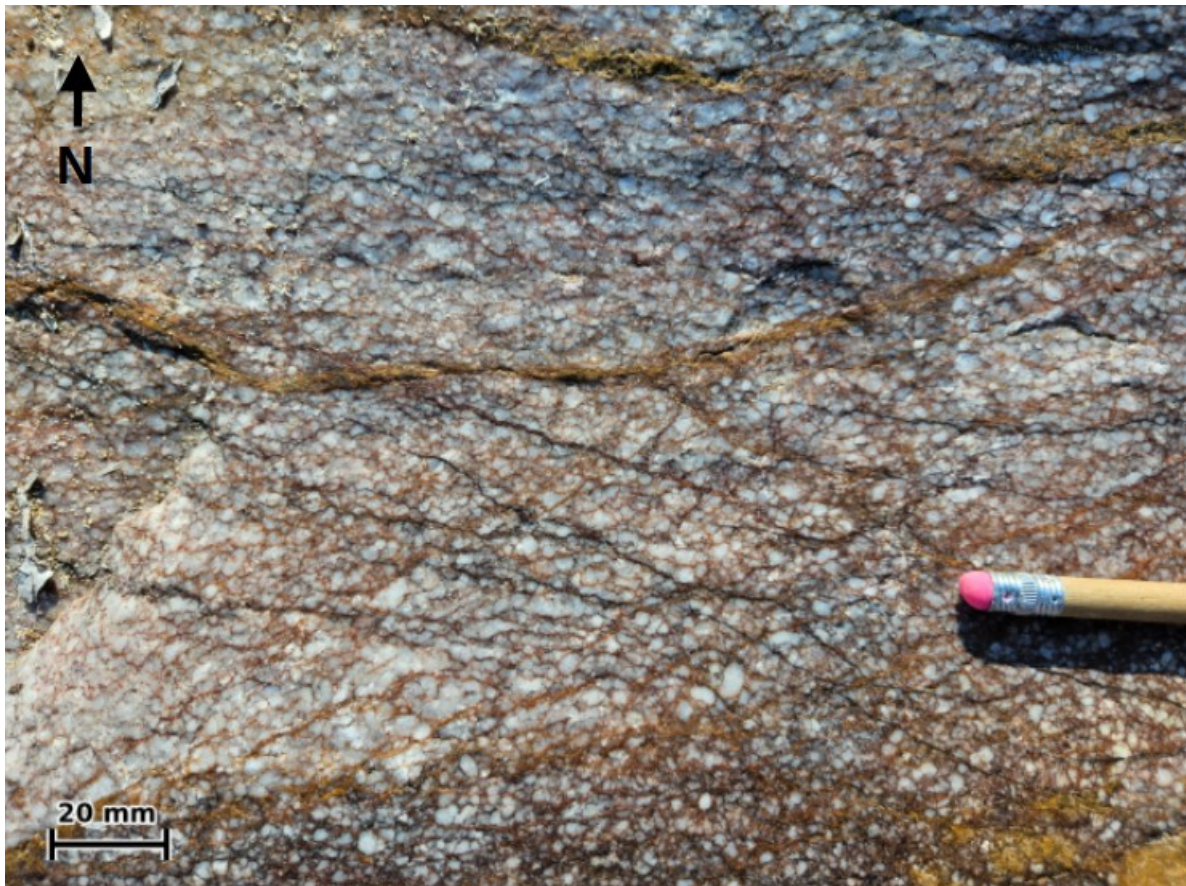
Figure 9. Close-up of fault breccia within the contact zone, showing strongly fractured and brecciated rock cut by darker deformation bands.
