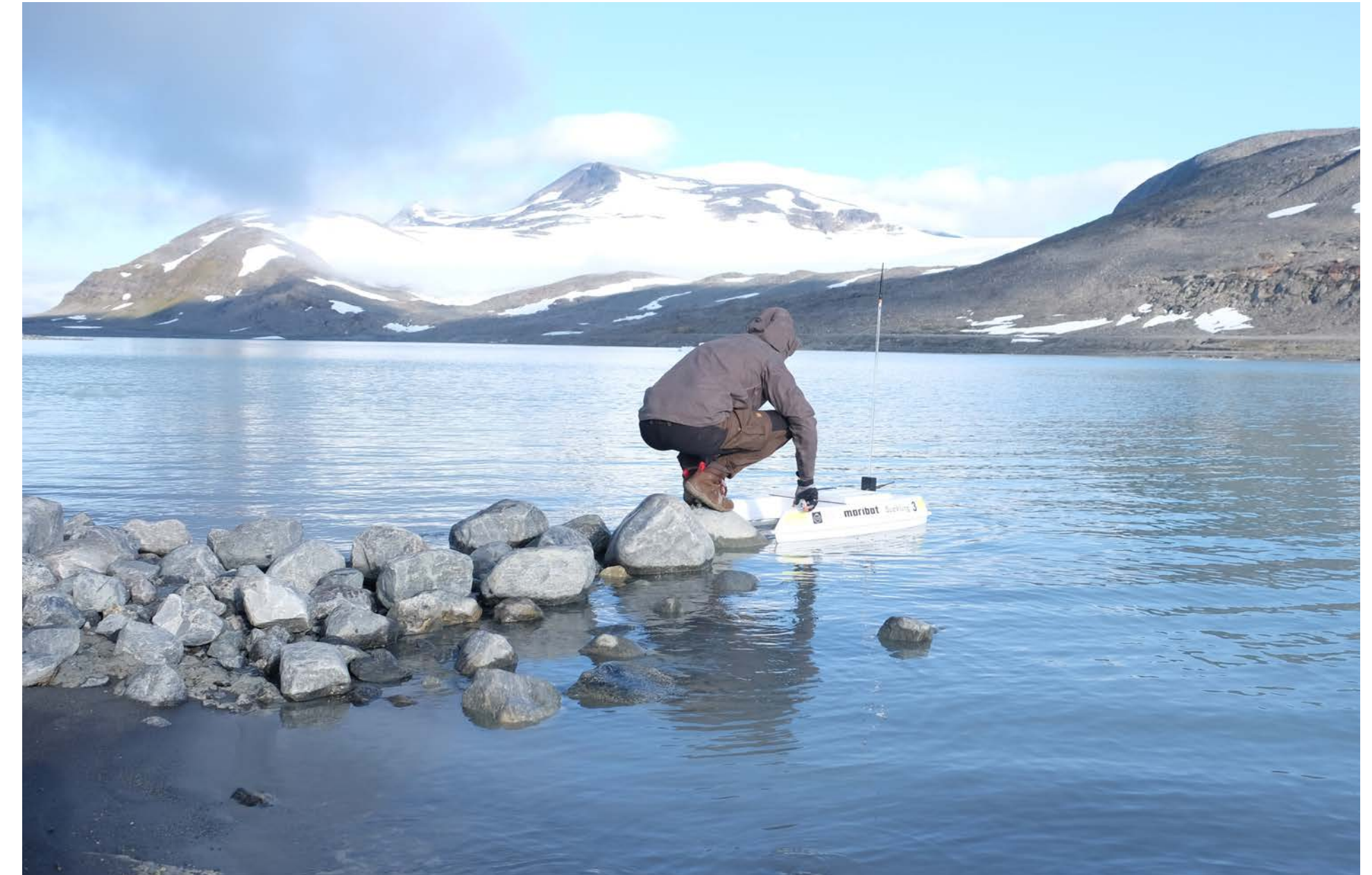
In 2019, the first mapping of the Sálajieгна glacial lake's bottom topography was carried out in a collaborative project between Stockholm University and KTH. With autonomous surface vessels called "Ducklings", the bottom was mapped using sonar. Photo: Nina Kirchner
