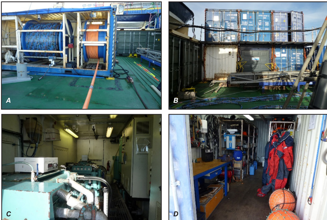
Figure GM-30: Containers on aft deck: (A) winch container; (B) compressor container (white), workshop container (blue) in the upper layer to the right; interior of compressor container: (C) and ; (D) interior of workshop container.
