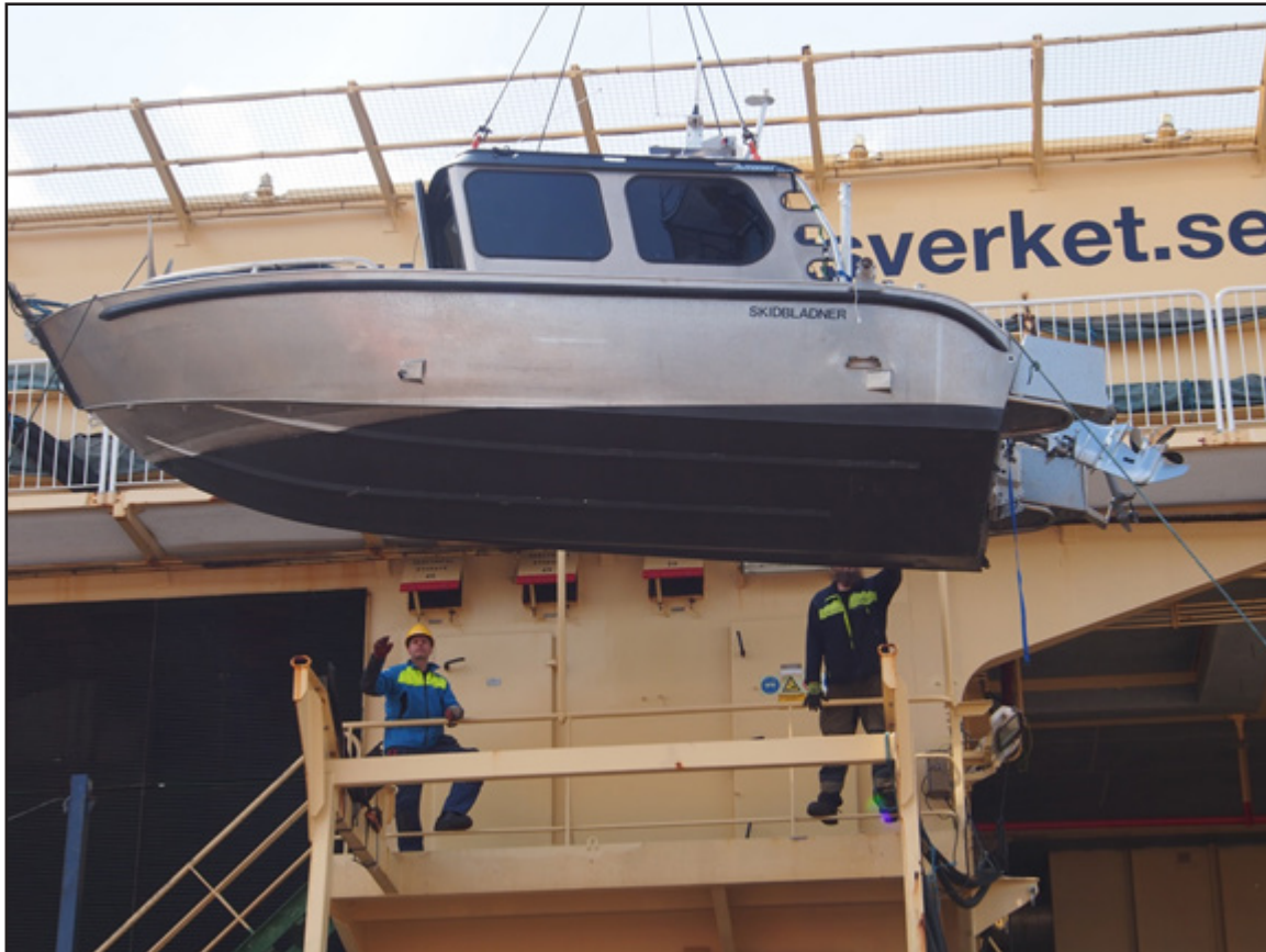
Figure GM-4: RV Skidbladner lifted onboard IB Oden in Landskrona, Sweden. The cradle normally used for Oden's workboat was used for RV Skidbladner during the expedition. Photo: Martin Jakobsson
