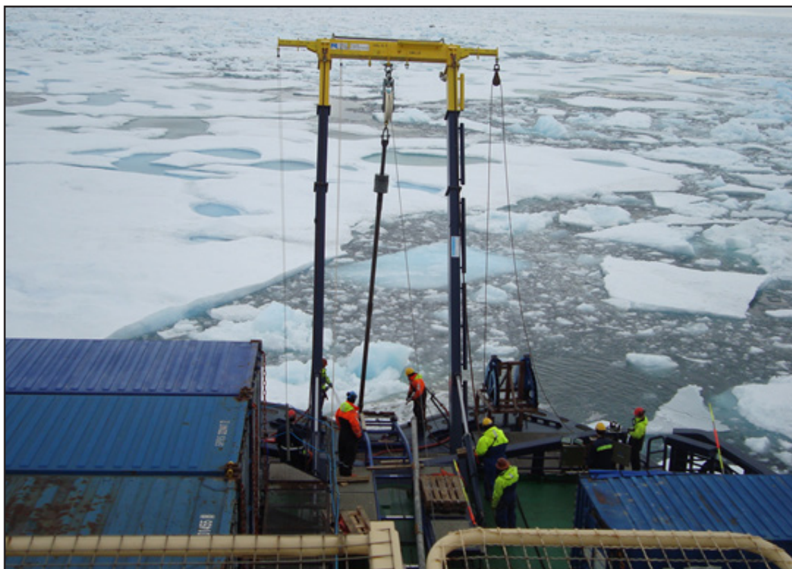
Figure SC-1: Gravity/Piston Coring System deployed from Oden 's A-Frame.
