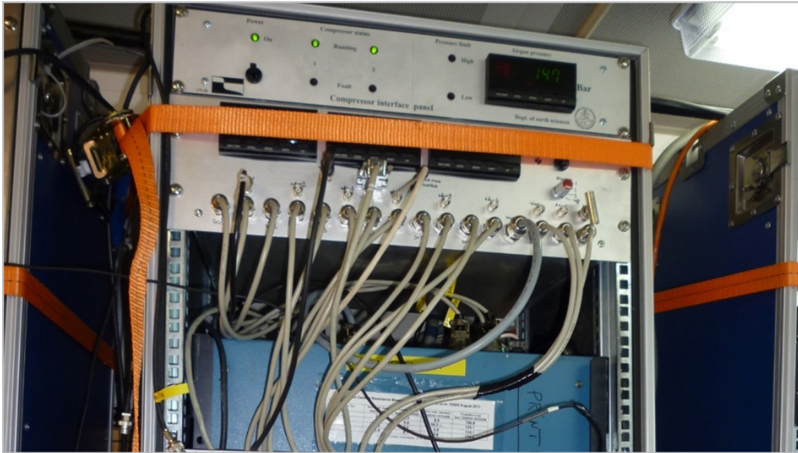
Figure GM-23: TGS-8 gun trigger unit and interface unit to umbilical (lower panel). Compressor monitor and air gun pressure (upper panel).
