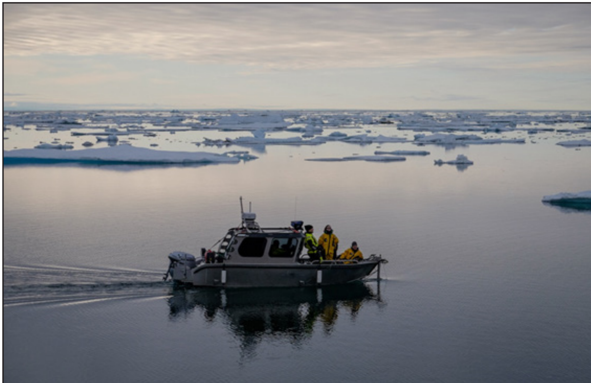
Figure GM-3: RV Skidbladner with the EM2040 bow mounted multibeam in operation. The multibeam and sub-bottom profiler (located on the port side, not seen on photograph) can be hoisted up for fast transit if required. Photo: Björn Eriksson
