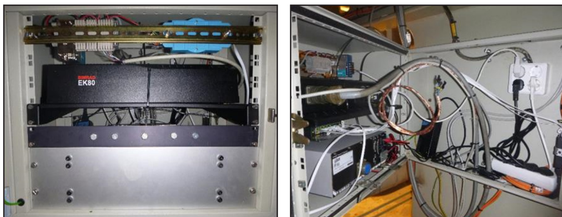
Figure WC-3: EK80 WBT installed in rack with EK60 GPT in tween deck below gym. Left – front view of rack with front door open – GPT is behind gray panel on bottom. Right – back view with back door open – GPT on lower level – WBT on upper level.
