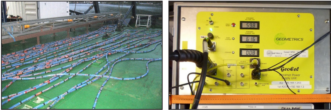
Figure GM-25: Geometrics GeoEel streamer on deck (left). Geometrics GeoEel streamer power supply unit SPSU (right).
