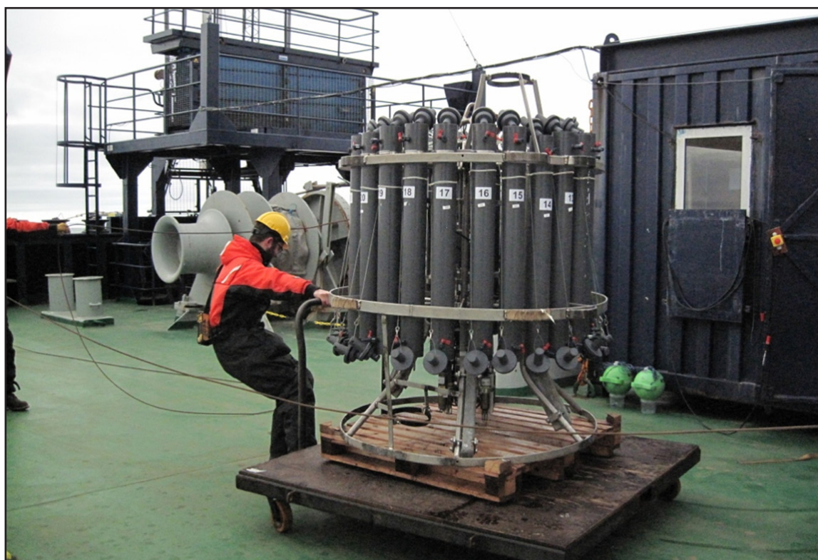
Figure PO-1: The University of Gothenburg SeaBird 911+ CTD system mounted inside a 24-bottle water sampling rosette.
