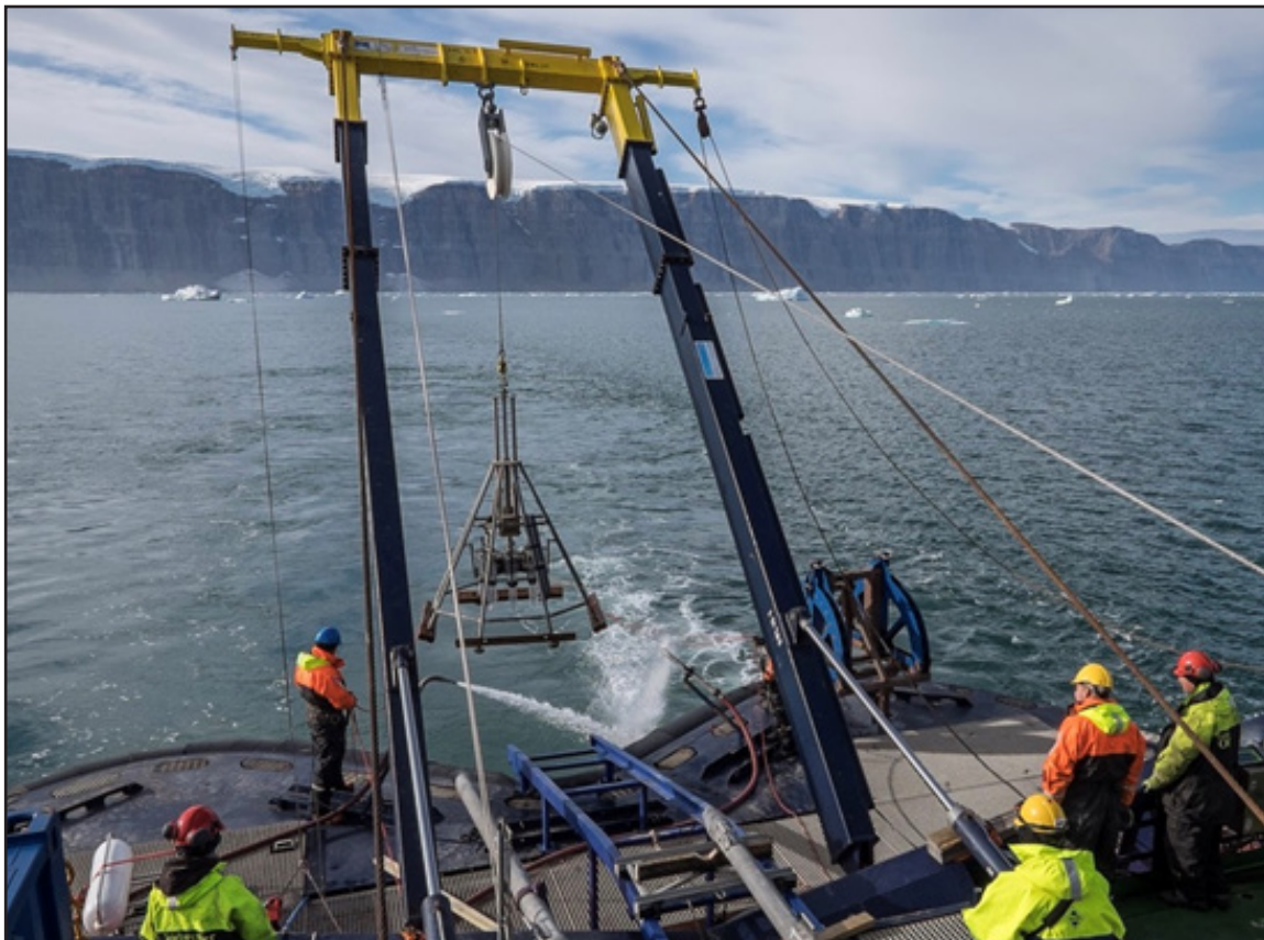
Figure SC-3: OSU Multicore system deployed from Oden’s A-Frame.
