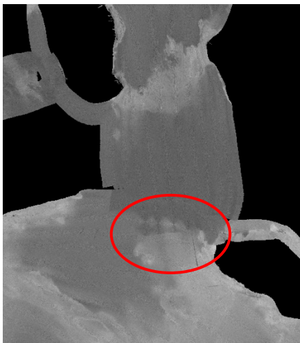
Figure 12. Screen-captured FMGT image showing data processing errors in the mosaic, circled in red. These boxy patches likely resulted from the joining of data from multiple surveys (with different backscatter intensity values for the same area).
