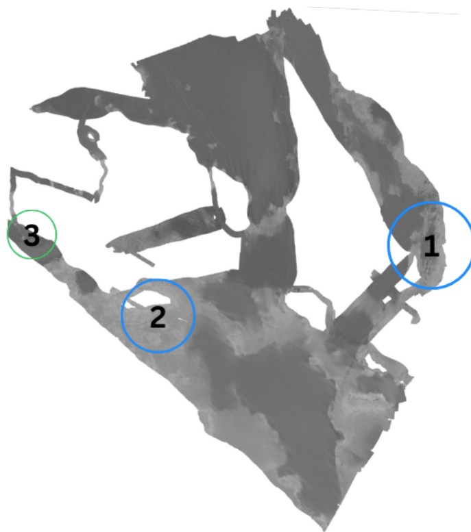
Figure 20. Landforms found on the seafloor, marked on BS mosaic. 1 indicates the region where terraces are found west of Fifång, and 2, those northeast of Askö. 3 Marks were pockmarks or gas seeps are found.
