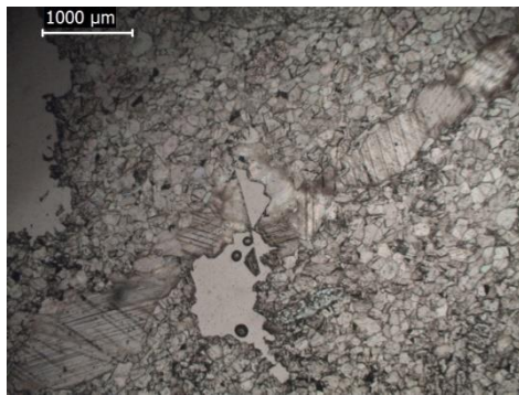
Fig. 20. Left (PPL) and right(XPL)- microcrystalline quartz matrix with visible calcite vein along the middle
