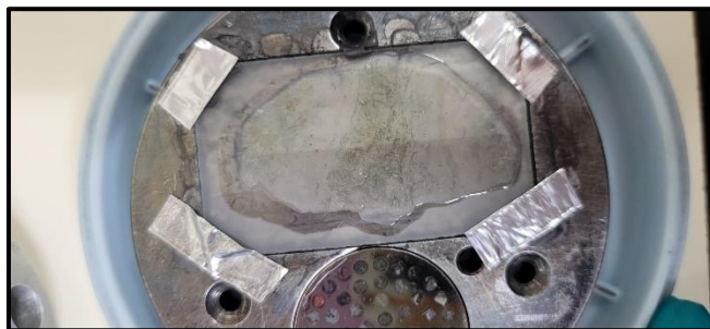
Fig. 8. Sample with half coating, aluminium taping and reference sample
