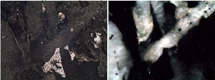
Typical texture of the sample. Loc 1, 25x, PPL and CPL.
