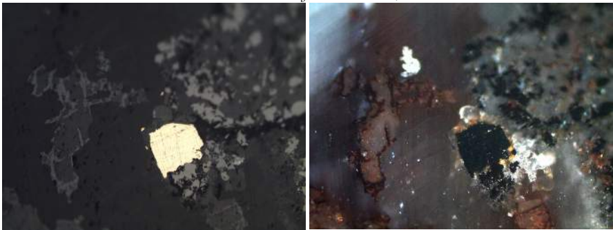
Pyrite being replaced by magnetite, small spots of brassy yellow chalcopyrite around and hematite with red internal reflection. 400x, PPL and CPL.
