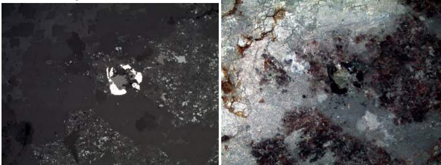
Ankerite with iron oxide rims. Loc.1, 25x, PPL reflected and CPL transmitted light..
