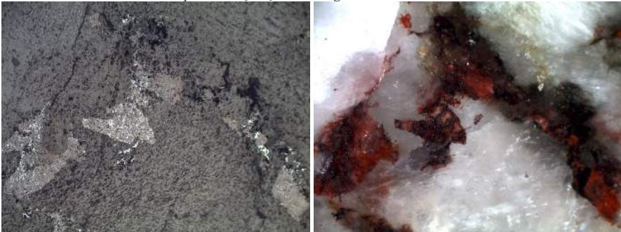
Hematite in the process of crystallizing? Loc.1, 100x, PPL and CPL.
