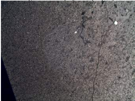
Large scale view illustrating the scarcity of the opaque phases. Loc.1, 25x, PPL.
