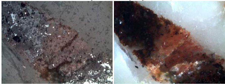
Iron oxides and red internal reflections in a crystal form. 400x, PPL and CPL.
