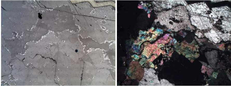
Ankerite with iron oxide rims. Loc.1, 25x, PPL reflected and CPL transmitted light..
