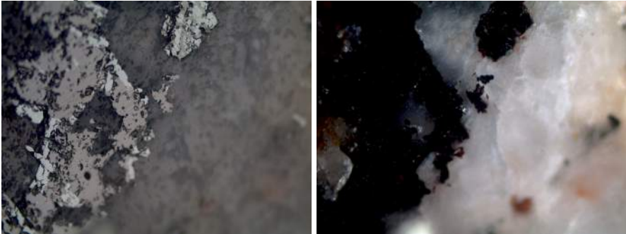
Magnetite and hematite in the rims in vicinity of loc. 1. 400x, PPL and CPL
