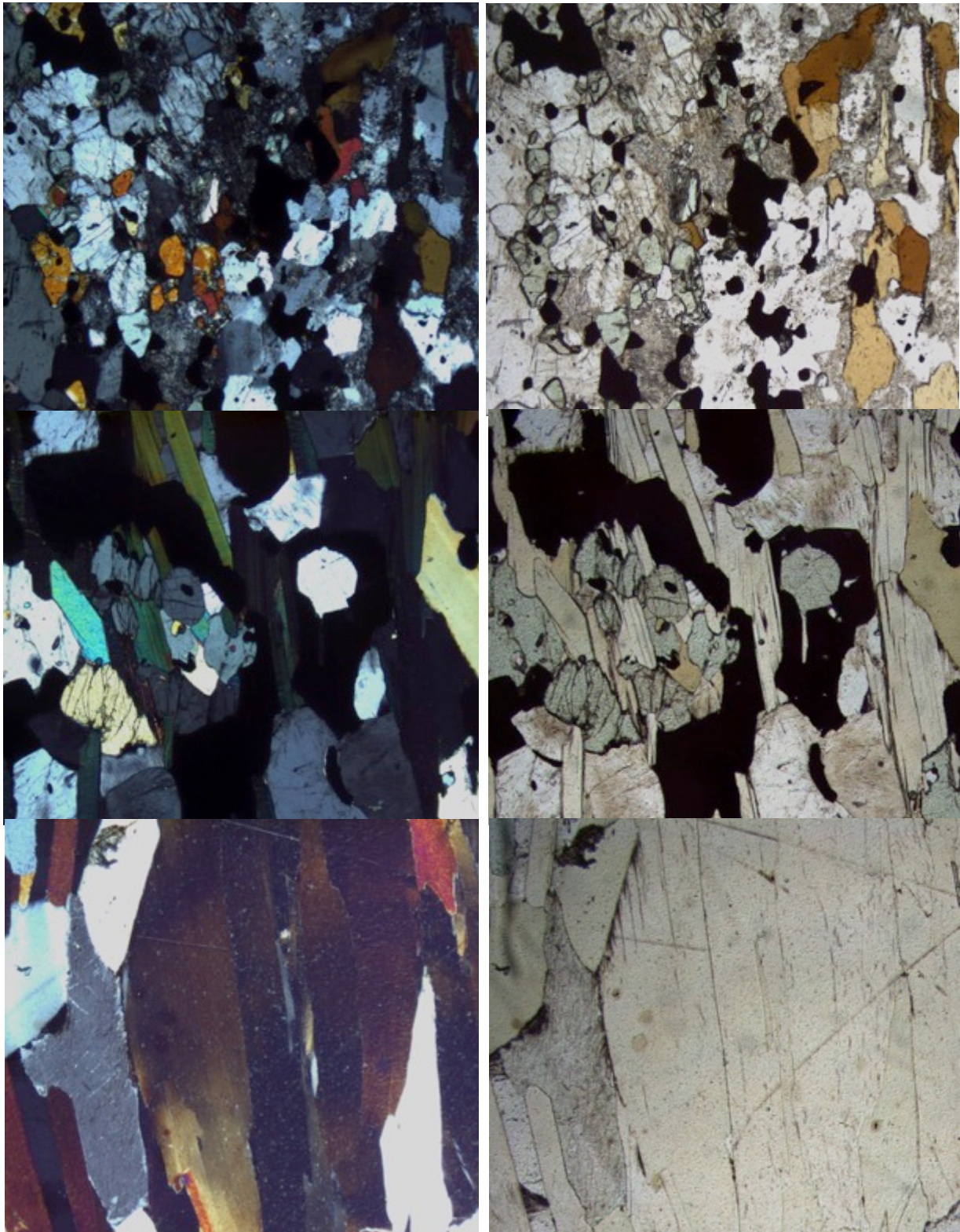
Fig. 17. XPL and PPL images. From top to bottom: GLE, GLE+Bt and BSF rock. A gradual decrease of felsic mineral content and crystal size increase is visible in the more altered rocks. Width of view 2 mm.
