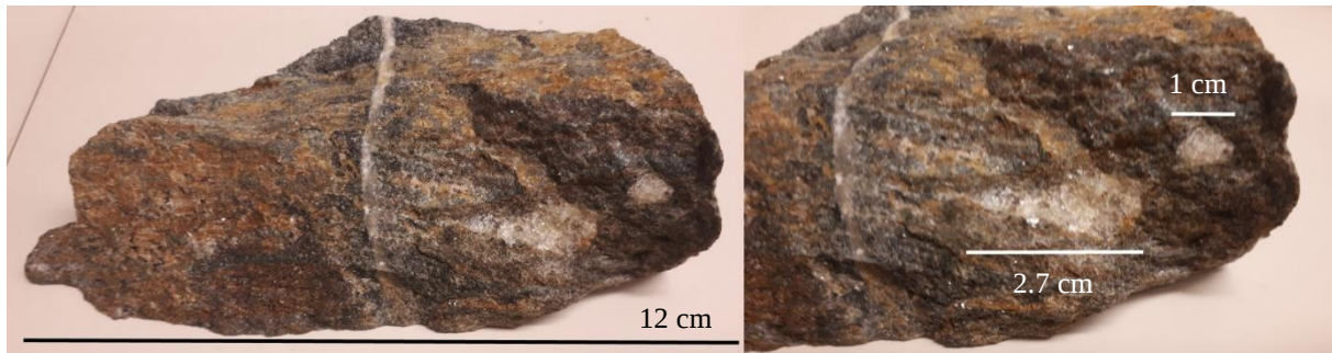
Fig. 21: Monomineralic patches of Qz on the weathered surface of sample SY-CM-03-blue.
