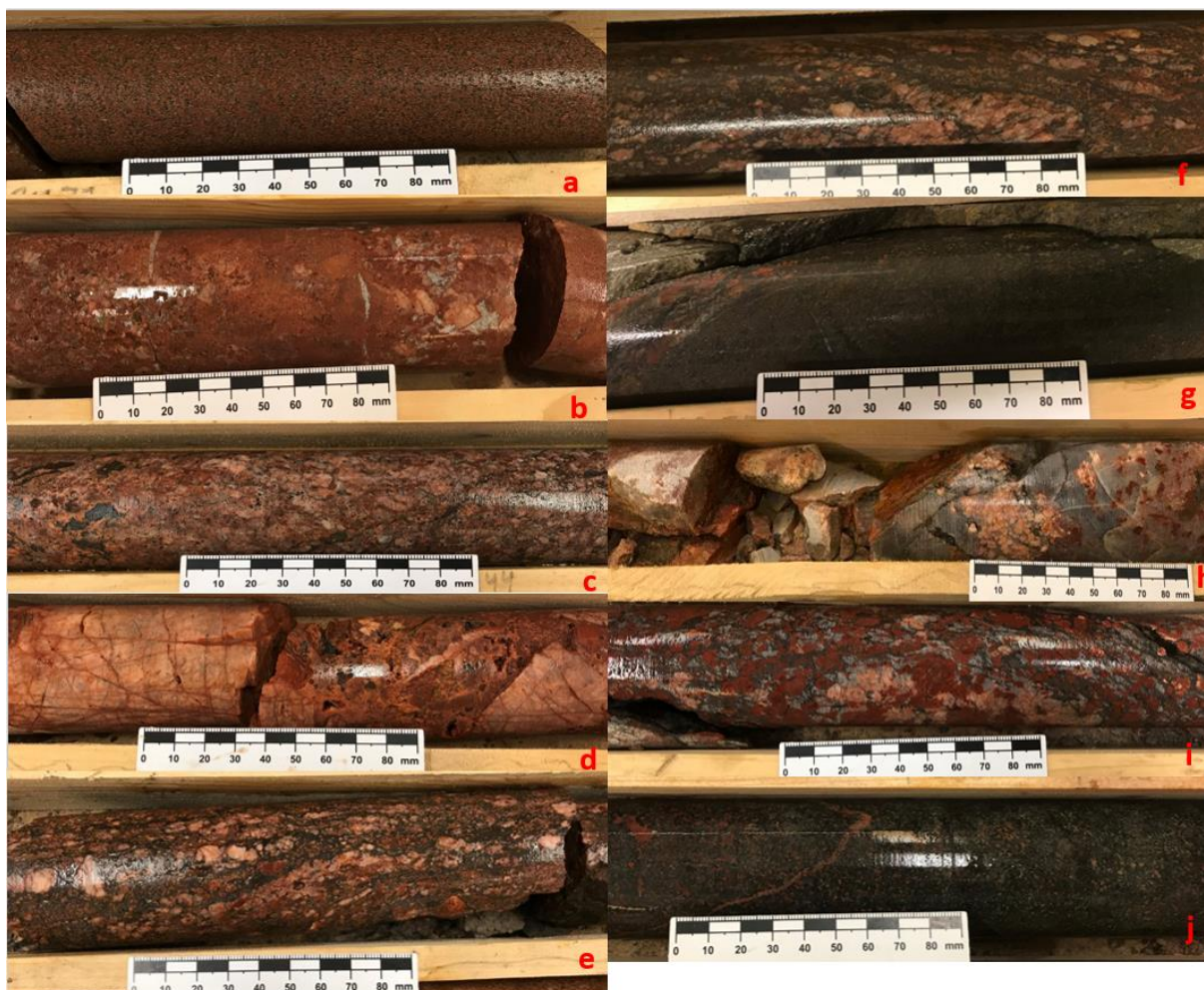
Figure 3 photo of the different rock and texture-types that was identified in the drill core.
