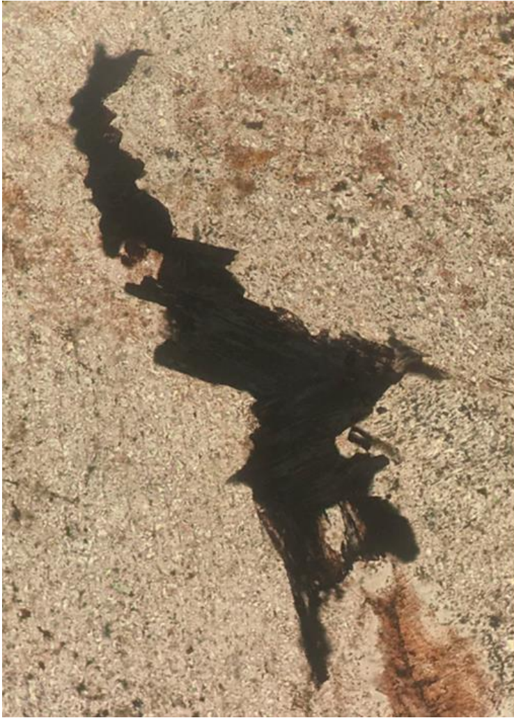
Figure 61 photo (X20) black fibrous mineral, tiny muscovite is present on the south edge.
