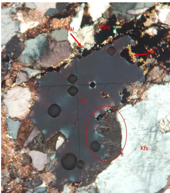
Figure 53 photo (X10) a vug and on the wall a k-feldspar that is overgrowth with a tooth shape mineral interpreted to be feldspar (adularia). Photo in xpl.
