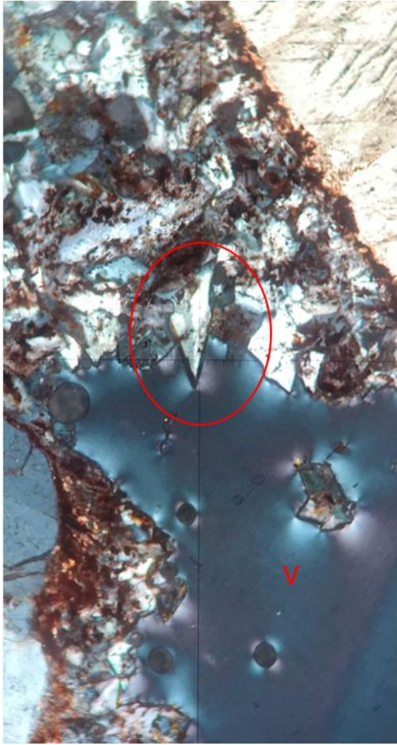
Figure 41 photo (X20) shows the vug wall where the interpreted feldspar with tooth shape. Photo in xpl.
