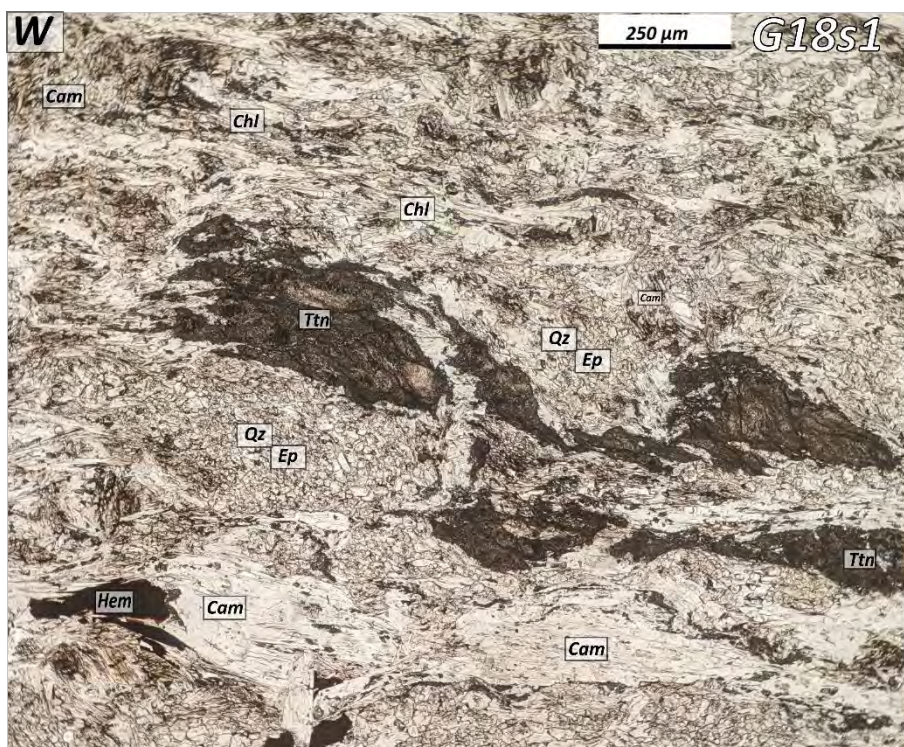
Figure 7 showing a foliation of elongated calcic-amphiboles, chlorite and titanite porphyroblasts. Rhombic calcic-amphiboles are situated as rotated grains amongst fine-grained epidote and quartz.
