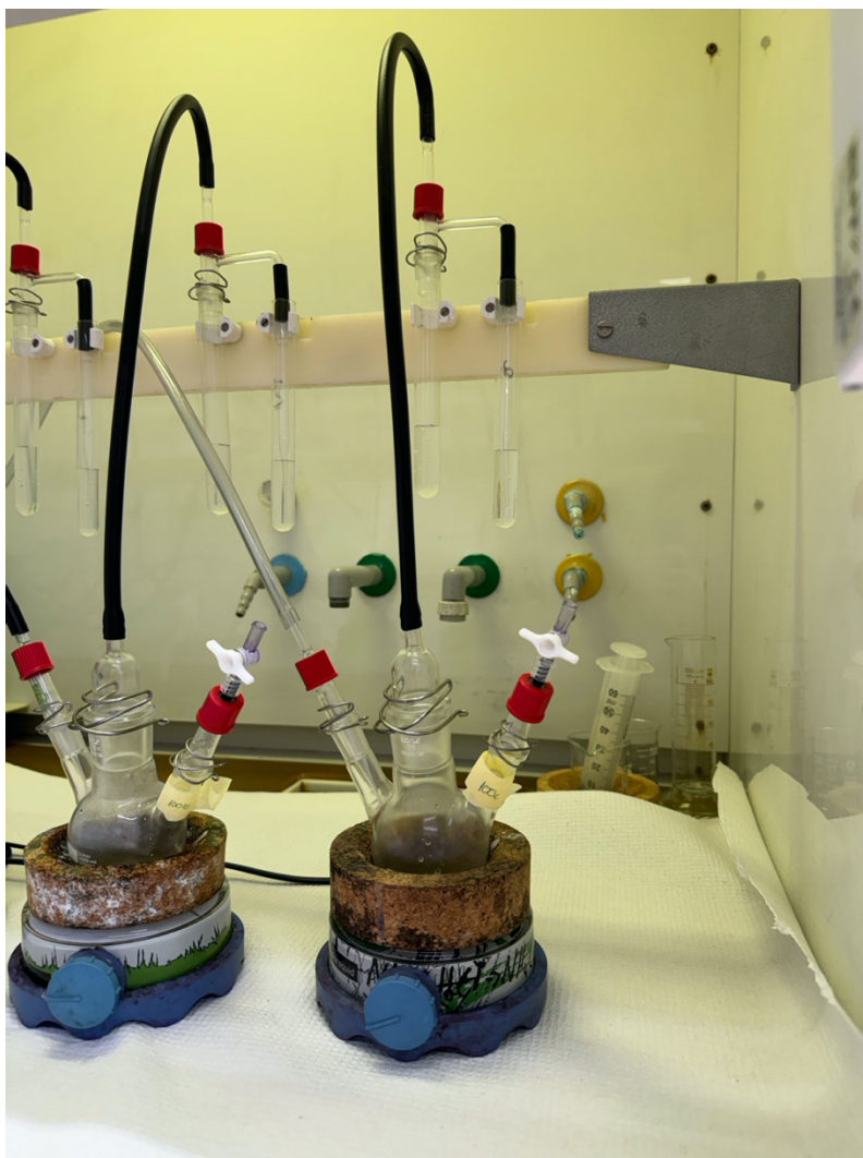
Figure 3. shows the three-neck distillation bottle. The left neck is connected to N_2 via a transparent tube. The middle neck is connected to the aerosol trap in the left test tube which is connected to the H_2S trap in the right tube. The right neck is connected to a valve where HCl and CrCl_3 is injected.
