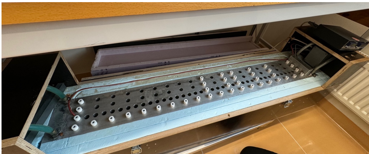
Figure 2. Aluminum temperature gradient block ranging from low temperature at the left side, to high temperature on the right side.
