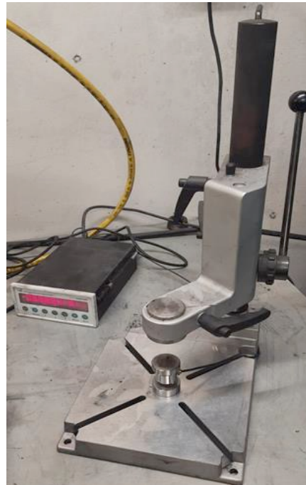
Fig. 10 STS: measures briquettes' splitting tensile strength.
