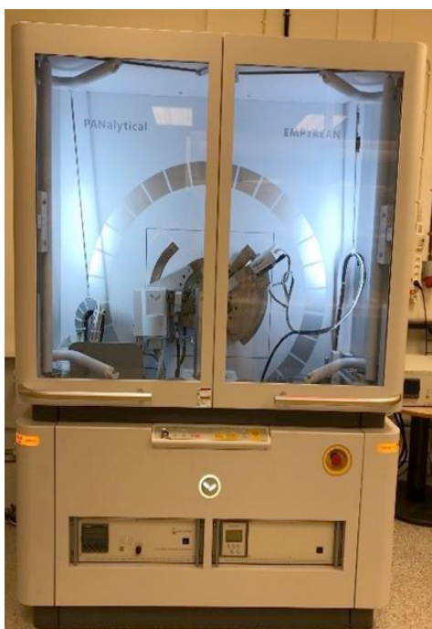
Fig. 13 XRD: tests phase composition
