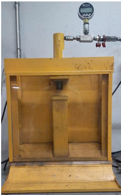
Fig. 9 Compression device: measures briquettes' strength.
