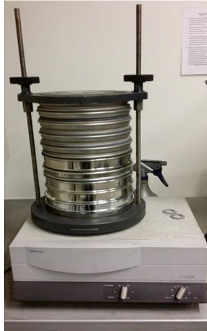
Fig. 8 Retsch Sieve Vibrator: measures the PSD.
