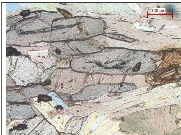
Fig. 17 Chloritoid with inclusions of rutile and graphite in matrix of white mica and chlorite (PPL).
