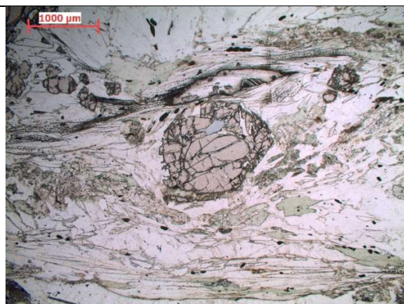
Fig. 11 Pressure shadow around garnet containing white mica, quartz and rutile (PPL).
