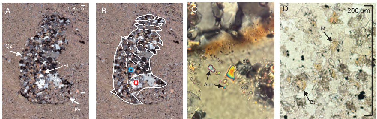
Fig. 36. A-C, XPL. D, PPL. A) Largest intrasedimentary pseudomorph in thin section 24EX12SEB, with discontinuous rim of quartz and pyrite. Full thin section seen in Appendix 1. B) Annotated version of A. Interpretations of internal shapes masked with dashed lines, based on direction of fringed terminations. C) Close up of red frame in B, inclusions classified as anhydrite. D) Close-up of area framed in blue in B. Bt = Biotite, with no distinct crystal shapes.
