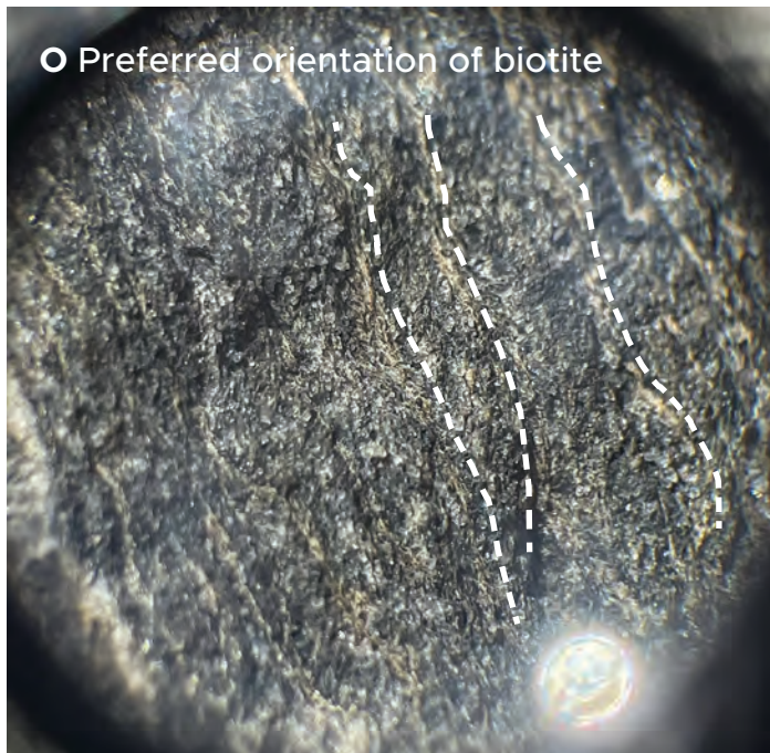
Figure 7 (continued) M Crenulation cleavage showing microfolding over an existing foliation is indicative of multiple deformation events during metamorphic conditions. N Close-up of crenulation cleavage. S_1 represents the earliest foliation, now folded into smaller crenulations. S_2 represents later foliation. O Preferred orientation of dark biotite and light mica crystals (marked with white dashed lines) with translucent quartz crystals within the foliation. The orientation suggests alignment of minerals along a foliation plane. The image taken through a \times 10 hand lens at Section 3A of the logged outcrop.
