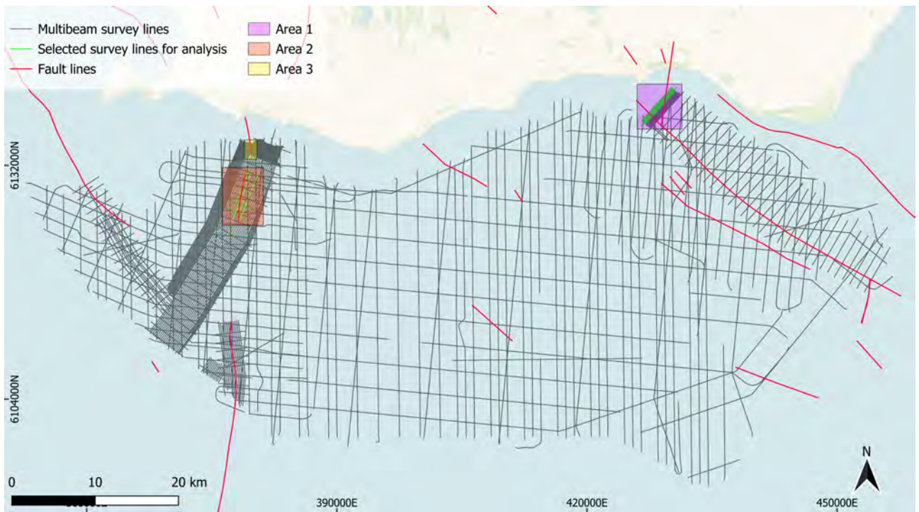
Fig. 14: Map over the CCS project area in the southwestern part of the Baltic Sea, just off the southern coastline of Skåne, Sweden. Marked on the map is all the MBES survey lines from 2023-2024, along with the documented fault lines. Also highlighted are the three sampled areas investigated in this report. Coordinate system: SWEREF99
