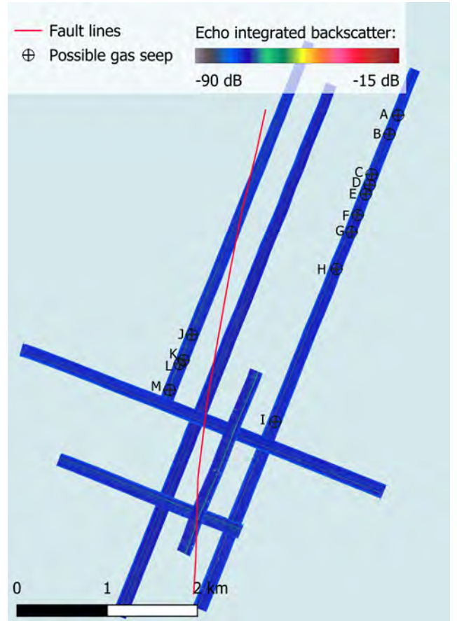
Fig. 28: Overview of the echo integrated grids created for Area 2, with labeled markers for any seep-like acoustic anomalies.
